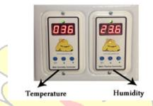
While the inside temperature is lower than adjusted value, the thermostat green light is on and when the temperature reaches to the adjusted value, the green light off.
