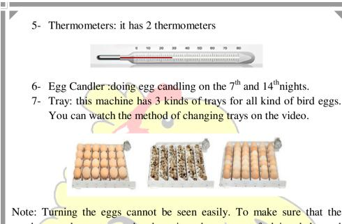
Note: Turning the eggs cannot be seen easily. To make sure that the gearbox works, put your hand on it and you must feel its shake and warmth.
