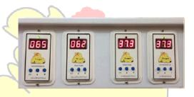
In normal situation main controllers work and set the temperature and humidity.
